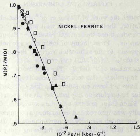
FIG. 6. Magnetization for 0.054 porosity (solid points) and 0.041 porosity (open points) nickel ferrite. The pressure variation is from 2 to 25 kbar.  $\blacktriangle$ ,  $\blacksquare$ ,  $\bullet$ ,  $\blacklozenge$ , and  $\times$  correspond to external applied fields of 45, 100, 325, 980, and 1960 Oe, respectively.  $\square$  and  $\circ$  correspond to 100 and 350 Oe, respectively.
