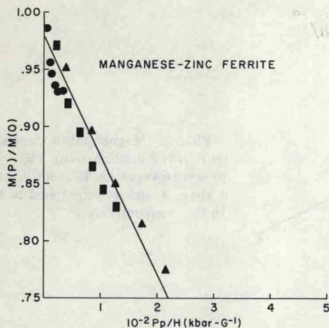
FIG. 5. Magnetization for 0.075 porosity  $\text{Mn}_{0.62}\text{Zn}_{0.25}\text{Fe}_{2.13}\text{O}_4$ . The pressure variation is from 2 to 12 kbar.  $\blacktriangle$ ,  $\blacksquare$ , and  $\bullet$  correspond to external applied fields of 35, 70, and 290 Oe, respectively.
