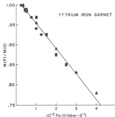
FIG. 4. Magnetization dependence on  $Pp/H$  for 0.02 porosity YIG. The pressure variation is from 2 to 20 kbar.  $\blacktriangle$ ,  $\blacksquare$ ,  $\bullet$ , and  $\blacklozenge$  correspond to external applied fields of 8, 16, 39, and 89 Oe, respectively.
